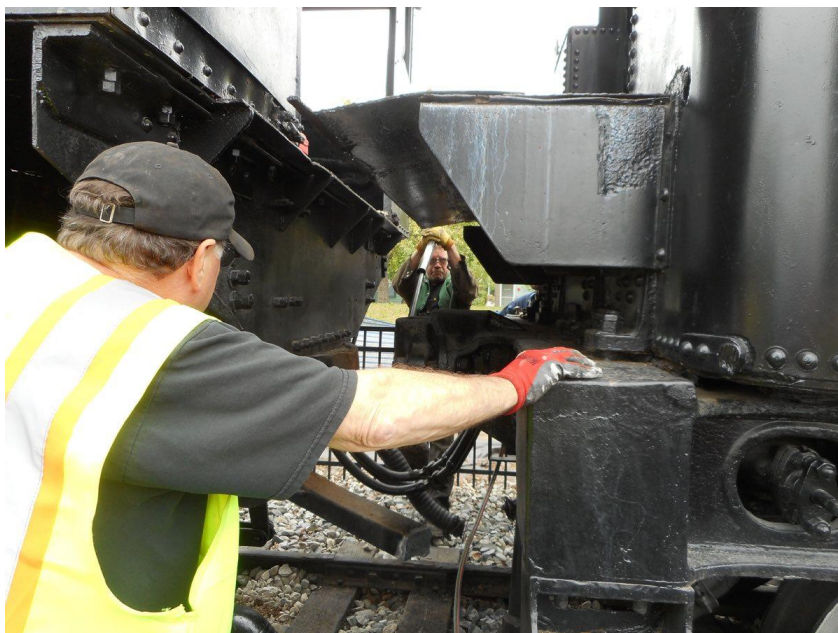
557 Maintenance Department volunteers remove buffer parts from ARR #556.
